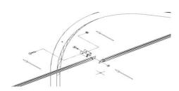
If your building has *cross ties* which are installed on the *purlin clip*, leave the *purlin clip* loose so that you will have a little more "wiggle" room for installing the *cross ties* later.
