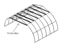
*Cross-ties* are an inexpensive way to reinforce your structure, typically increasing the snow/wind load by 5 pounds per sq. ft. They are made from the same material as the *purlins* and *wind-braces* and, depending on the width of the structure, between 10 and 14 feet long. In cases where the *cross-ties* are not included in the package they are available as add-ons.
