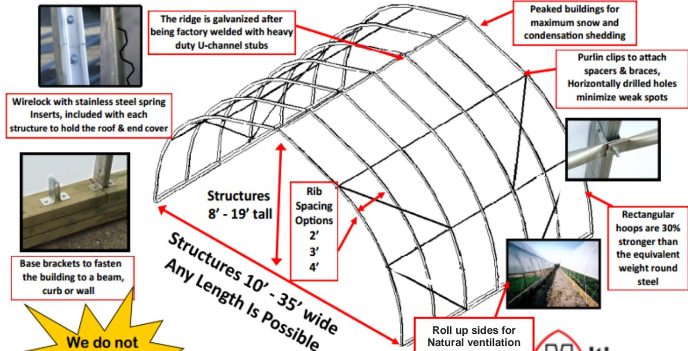
Wirelock with stainless steel spring Inserts, included with each structure to hold the roof & end cover
